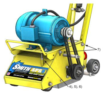
7. Loosen (do not remove) the four bolts(2 per side) that secure the motor mountplate to the main machine frame.
