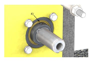
5. Remove the bearing assemblies on both sides on the machine using the 9/16" socket
