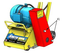
4. Lubricate the motor plate (belt tensioning) jackscrew with WD40 on the front left of the machine.
