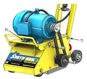
10. Roll the new belt on one groove at a time (two or single multi-groove belt) on both the top and bottom pulleys.
