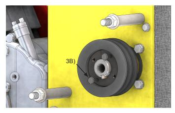
4. At this point the shaft driver must be removed using the C-clip removal pliers for the retaining ring and a 5/32" hex key for the 2 set screws.
