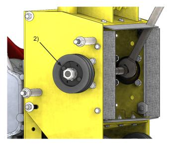
3A. Remove the remaining 3 screws using the 7/16" socket and insert them by hand into the 2 threaded holes as shown below (3B)
