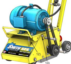
14. Now from the front of the machine observe the motor plate to machine alignment. Tightening the belts with the jackscrew tends to cause the right side of the motor plate to lift higher than the left side. By pushing down on the right front side you can level the plate and then tighten the front right screw to secure in a level position.
