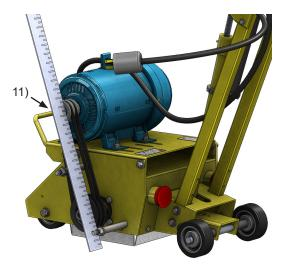
12. After installation, use the 3/8" open wrench to screw out the belt tensioning jackscrew under the motor plate to tension the belts to your desired tension. Do not over-tension the belt.
