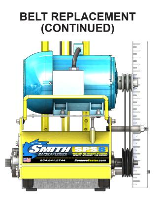
15. Now tighten the rear securing bolts with the two 9/16" wrenches.
