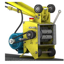
3. Once the hex nuts are off you can slide the shaft off towards the sideplate side of the machine and the drum will fall out. (use precaution as it is HEAVY)
