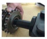
Slide felt washer onto the shaft into the space between the cutter edge and the bearing edge.
