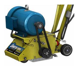
18. Replace the belt cover using the 3/4" box wrench.
