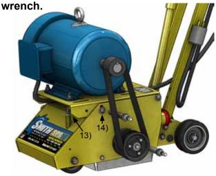
15. Now from the front of the machine observe the motor plate to machine alignment. Tightening the belts with the jackscrew tends to cause the right side of the motor plate to lift higher than the left side. By pushing down on the right front side you can level the plate and then tighten the front right screw to secure in a level position.
