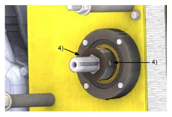
5. Remove the bearing assemblies on both sides on the machine using the 9/16" socket
