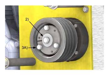
3B. Once all 3 screws are in, begin to turn them using a socket and do so EVENLY to allow the bushing to back out smoothly. Once the bushing is out, remove the pulley and key.
