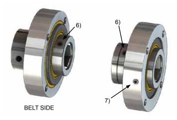
7. With the hex bushings out, the remaining bearings and housings are the same. To remove the bearing from the housing, use the 1/8" hex key to remove the set screw on the housing and tap out the bearing using a mallet
