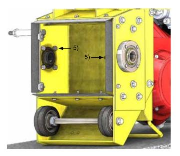
6. At this point remove the hex bushings from the bearing assemblies (note that the belt side bushing is much thicker and has holes for set screws) using the 5/32" hex key
