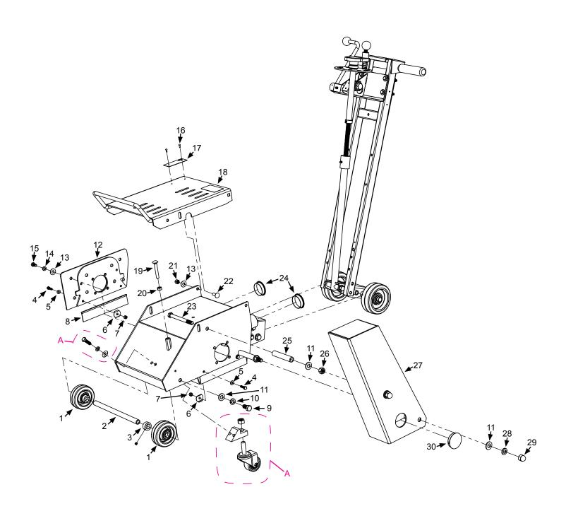
SPS8.WPKA - SPS8 ESSENTIAL WEAR PARTS KIT: Includes a set of 4 wheels, dust skirt with guards, vacuum cap, a set of handle grips, a hex drive shaft, a set of 2 left handed jam nuts, and a set of 3 cap screws for shaft driver (65028)
