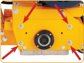
Remove sideplate and insert drum. When drum is installed, replace sideplate.
