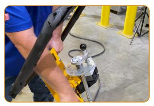
Machine requires a minimum 50A circuit and is 220 single-phase. If running on a generator, it must have MINIMUM 11k CONTINUOUS power, not 11k MAXIMUM. Low power could result in overheating and burning out the motor.
