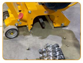
PCDs, diamonds, and milling cutters are DIRECTIONAL; they can only go forward. Improper installation will result in severe damage to the cutters.
