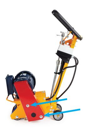
Remove red cap on either dust port to attach a vac system. -
