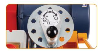
Set depth by lowering the handle, dialing the drum down until the cutters touch the surface, then raise the handle and dial in your cut depth. When lowering the handle to cut, use care that the machine doesn't pull the operator forward. The operator MUST hang on to the machine.
